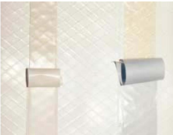
**Fig 1C: Detail showing butyl double sided tape and Polyseal tape**
